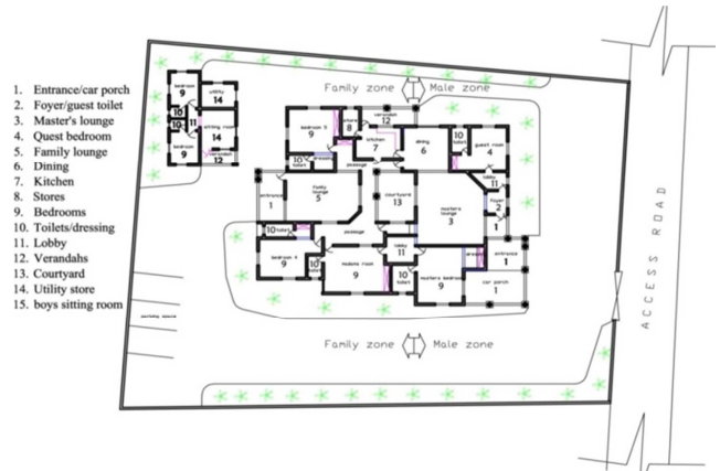
Figure 5. Postmodern residential plan showing cultural sustainability issues with regard to zoning and privacy aspect. Designed by Zailani and Sa'ad Raji, Source: Delammed Interprise 2010.
